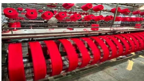
Machinery Name: Reeling machine
