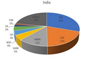
Technology-wise distribution of different WWTPs based on installed capacity:
