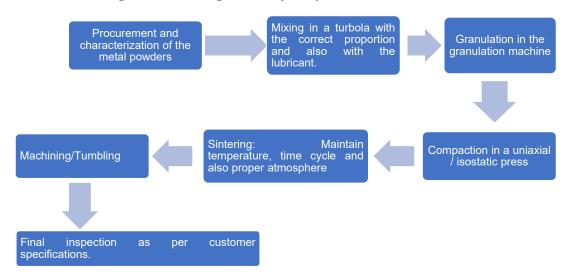
Tungsten Heavy Alloy is an alloy of Tungsten, Nickel and Iron/Copper. The percentage of tungsten in the alloy generally varies from 90-95% depending upon the application and the balance is Nickel and Iron/Copper in the ratio of 7:3.
