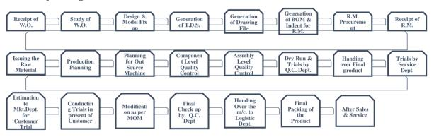
Our process for manufacturing machines starts after our marketing and sales team finalizes the machine dispatch schedule with the customer. Thereafter, the material requirement planning is calculated, following which the parts delivery schedule is sent to relevant suppliers and in-house manufacturing unit.
